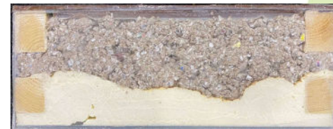
Top Down View of Air/vapor Sealed Wall Chamber with SPF and Cellulose
